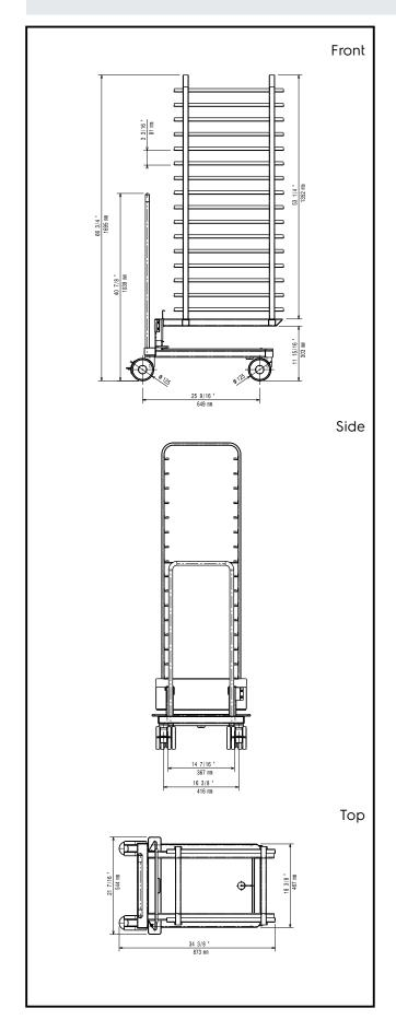
Cooking accessories Bakery/pastry trolley with rack holding 600x400mm grids
